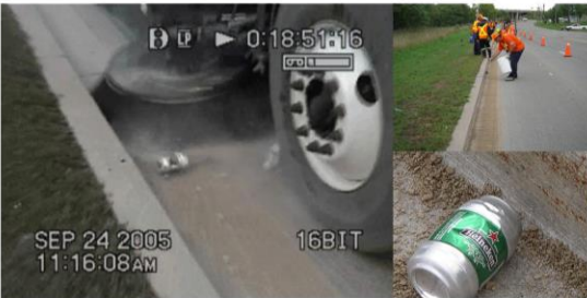
Section D - Pick-up of Large Debris (l: 30m X w: 2m)
