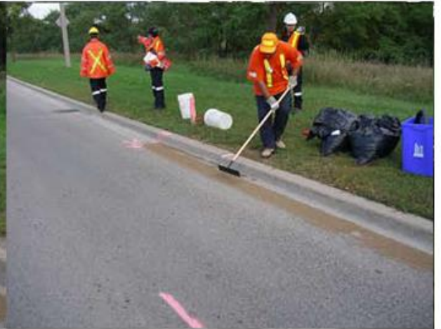
(iii) Raking the Standard Test Material Towards the Curb
