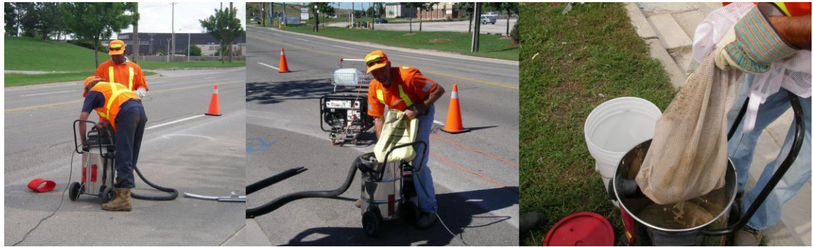
Figure 10 Shop-Vac cartridge, HEPA filter bag, and cheese cloth
